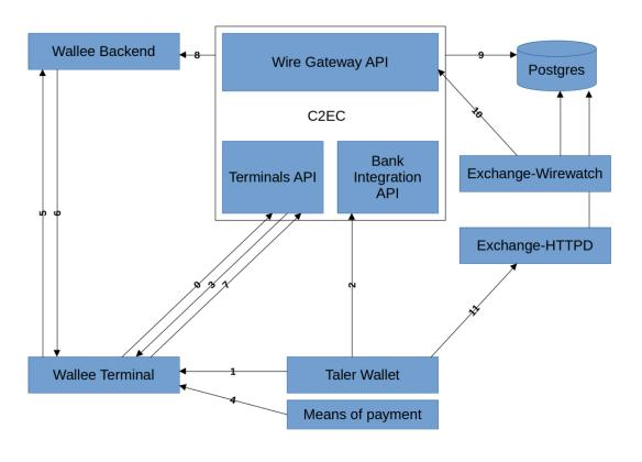
Figure 2.2: Diagram of included components and their interactions
